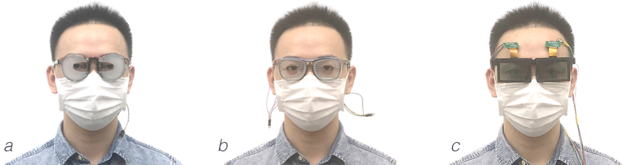
Figure 1: a) Dynamic Peripheral Vision Blocking Glasses. b) Saliency Reducing Glasses. 3) Gaze Guiding and Saliency Adjustable Glasses.
