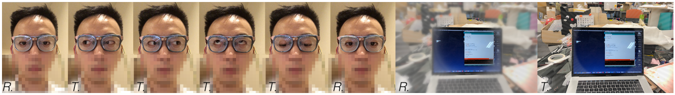
Figure 5: Saliency Reducing Glasses Wearing Demonstration. R. indicates Saliency Reducing Mode. T. is Transparent Mode.
